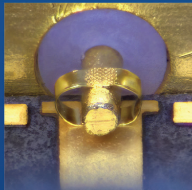
Omega wrap (Double-C) ribbon bonds on feedthroughs
