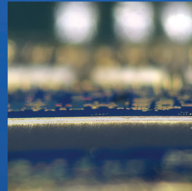
Conductive epoxy die attach bond lines as thin as .002"
