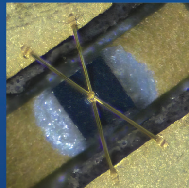
Cross bond stitching on ultra-small mesa diodes
